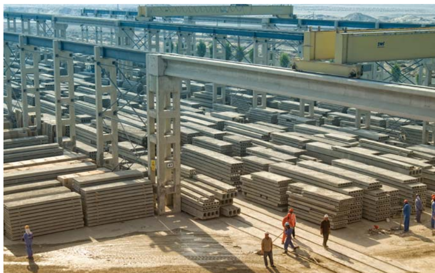
Storage area in the hollowcore factory.
