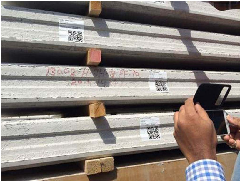
Bar coded Hollowcore slabs leaving the factory ground
