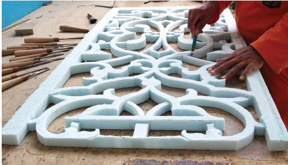
Prototype of counter-mould in polystyrene.
