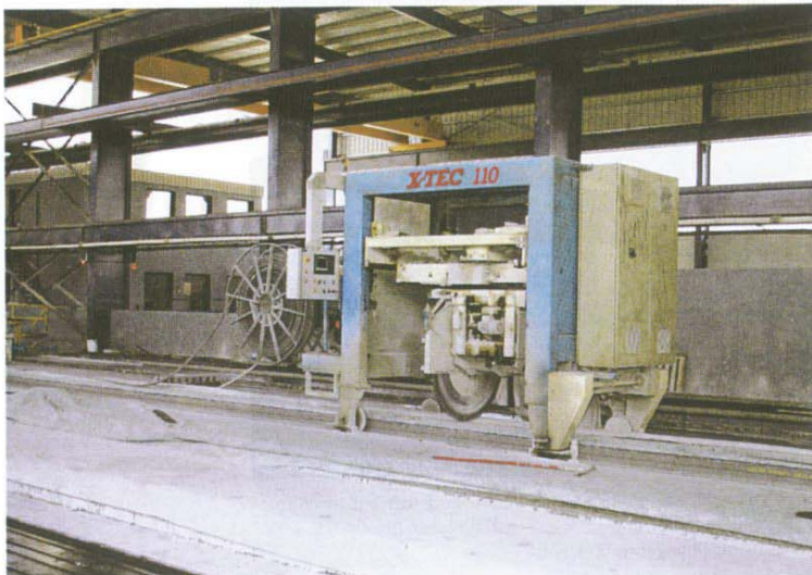
Hollow core saws of type X-Tec 110 are used for cuts from 0 to 180°.
